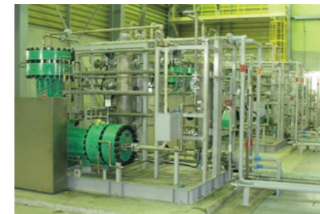
水素ガス圧縮機 処理量:200Nm 3 /h, 300Nm 3 /h, 500Nm 3 /h Hydrogen gas compressor Processing Capacity: 200Nm 3 /h, 300Nm 3 /h and 500Nm 3 /h
